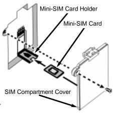
Figure 6 - Mini-SIM Card Installation.
